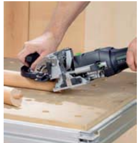
Joining round poles with the handrail fence.
