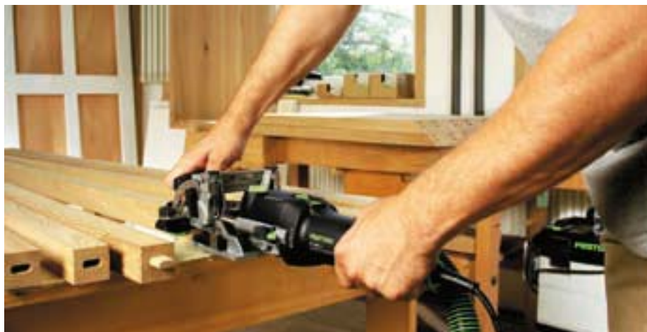
Useful accessories making working easier: by using a special stop, narrow strips of wood can be aligned without problems, even for mitre cuts.
