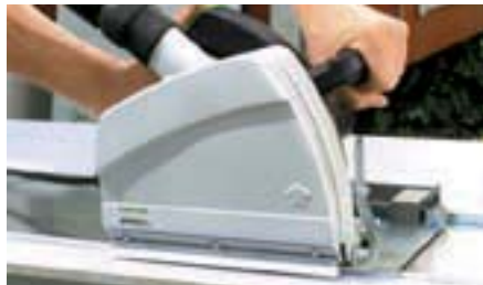
A closed extraction hood and sealing brush for maximum dust extraction.
