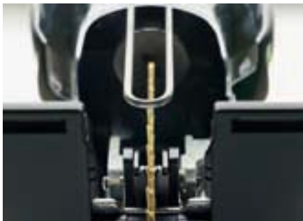
The CARVEX guidance jaws adjust automatically to different saw blade thicknesses.
