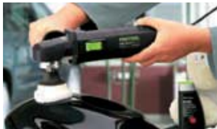
The RAP 80.02 E is ideal for small, curved surfaces, eg a motorcycle tank.
