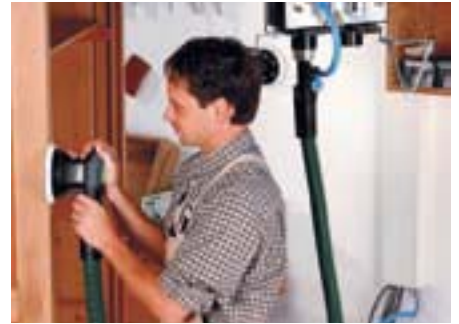
LEX 2 eccentric sanders are also suitable for work on vertical surfaces because of their low weight and excellent manoeuvrability.
