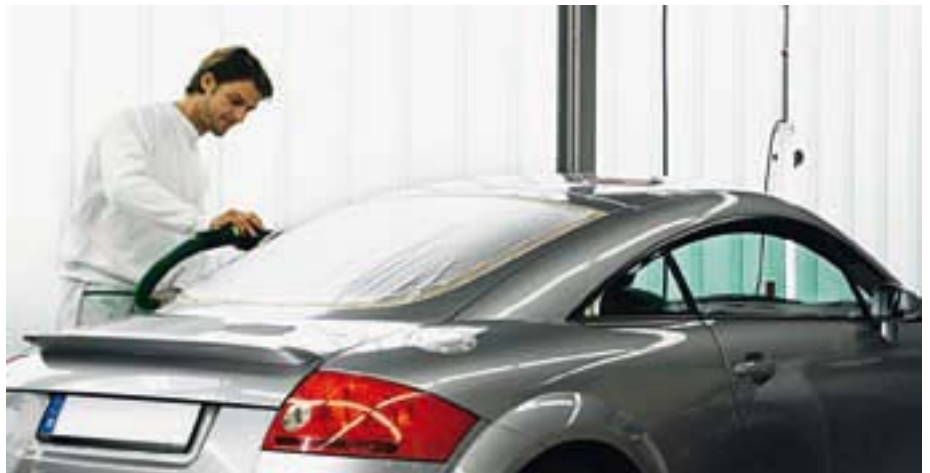
Specially developed for the workshop: the LEX 2 eccentric sander and the IAS 2 system with mobile dust extraction.
